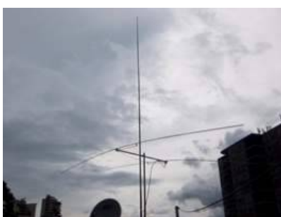
28MHz HB9CV、HF Vertical
